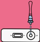
Apply 3 drops of sample to the sample port of the test cassette. Squeeze the bottle gently for controlled application.
